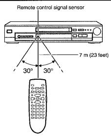
Aim at the sensor, avoiding obstacles, at a maximum range of 7 m (23 feet) directly in front of the unit.
